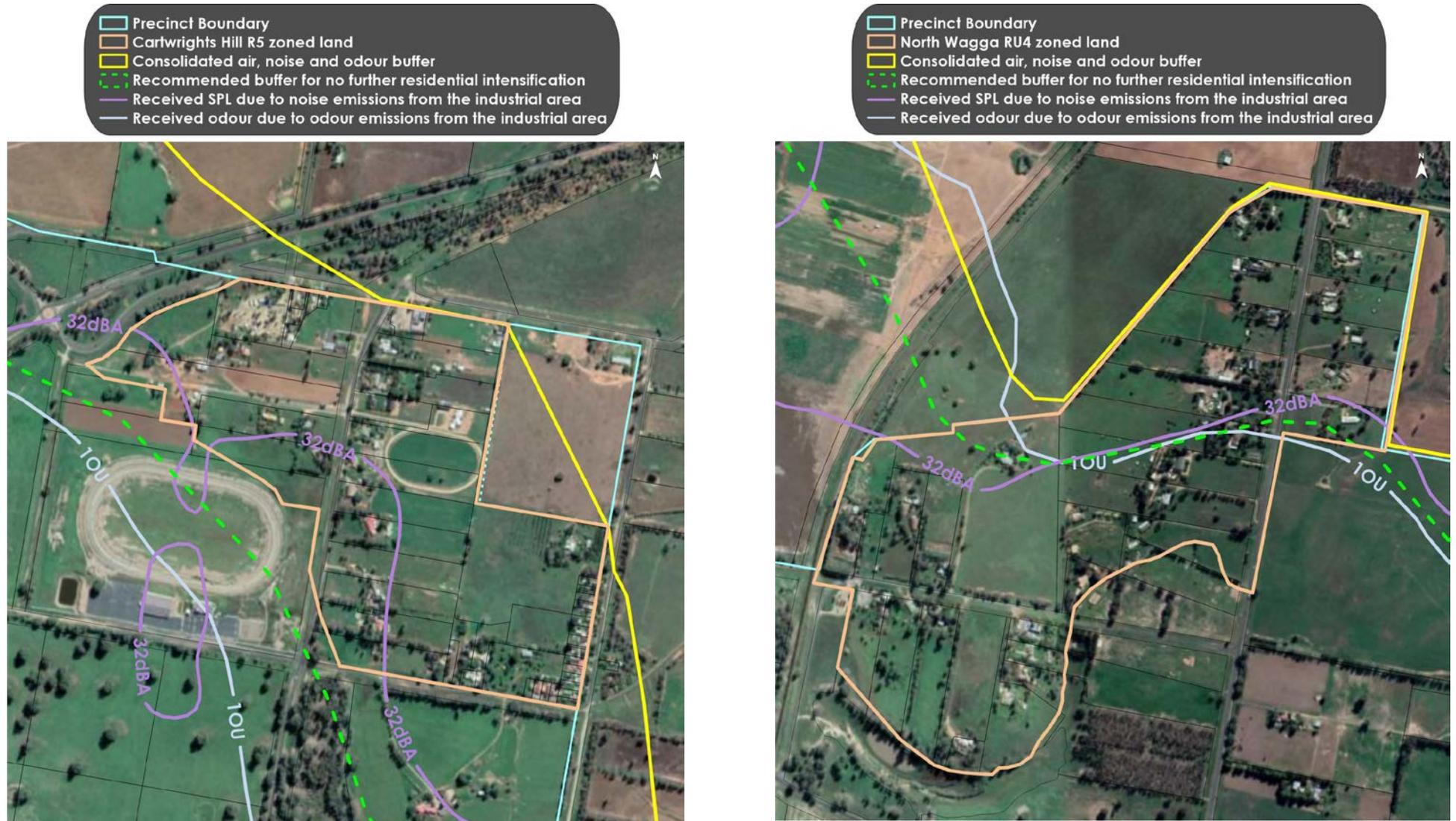
Figure 8-2: Recommended buffer for minimising residential intensification
