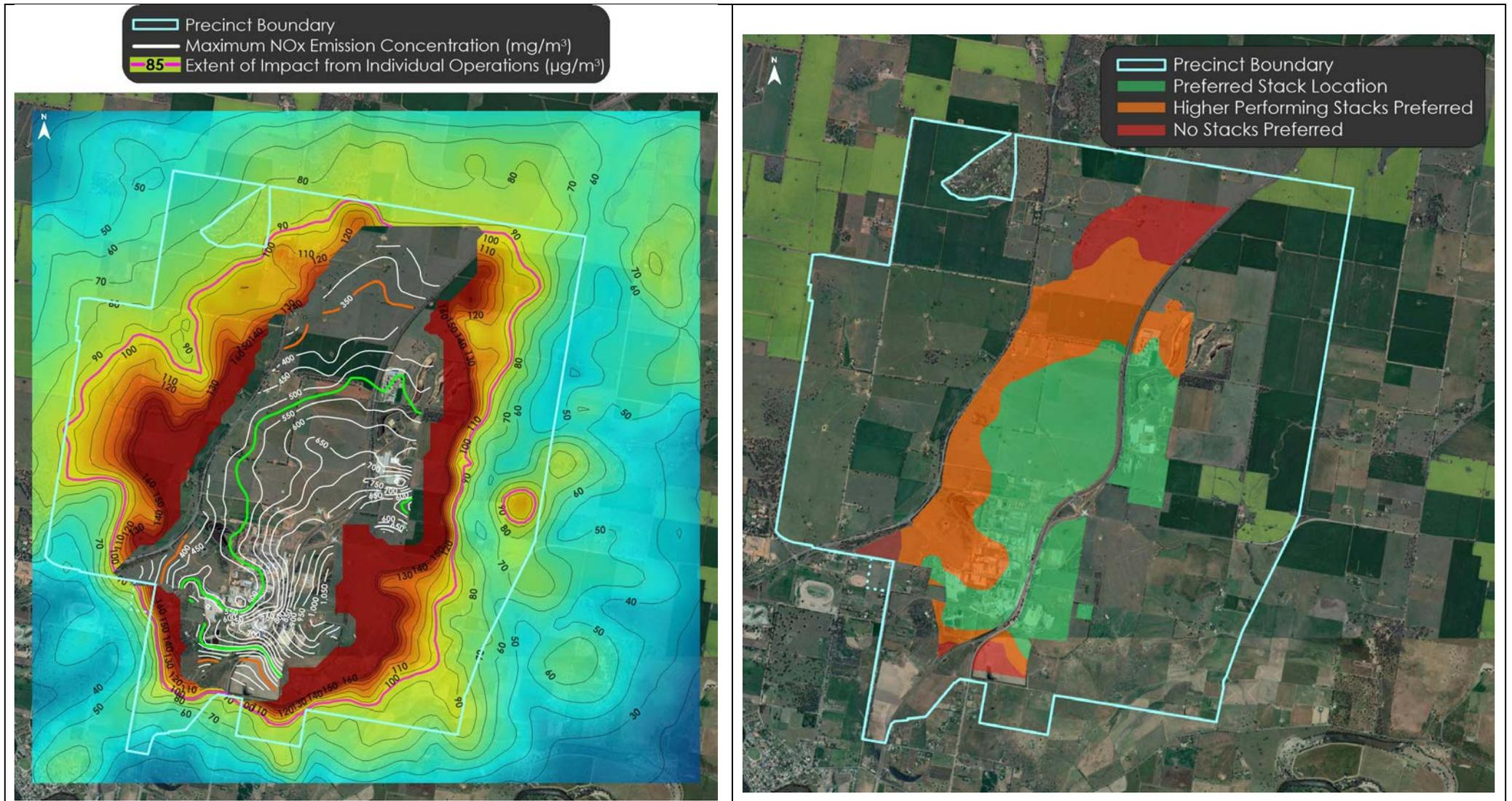
Figure 7-3: Example of Air emissions rate per stack (left) and received air pollutant concentrations (right) due to NO<sub>x</sub> emissions from the industrial area
